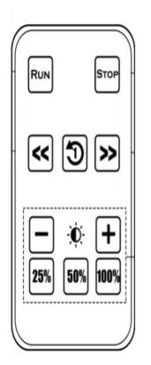
Run: turn the device from 'stand-by' to 'running'
