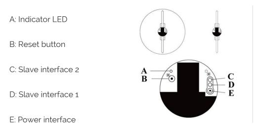
Power interface: use the AC adapter to supply power ,Slave interface: used to connect to slave devices.Reset button: switch between master/slave modes; pair with remotes.Indicator led: indicating power supply, on/off, modes, etc.
