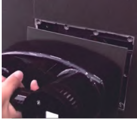
Use the sucking tool to pull the module away from the cabinet.
